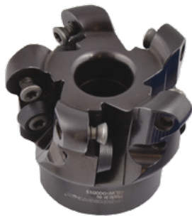
GLW-000015 J-groove R8 milling head (5 inserts R8 required)
