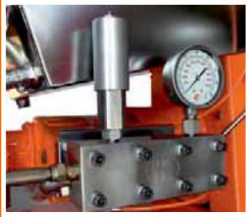
Stainless steel pump-head. Integrated cooling for plunger-seals.
